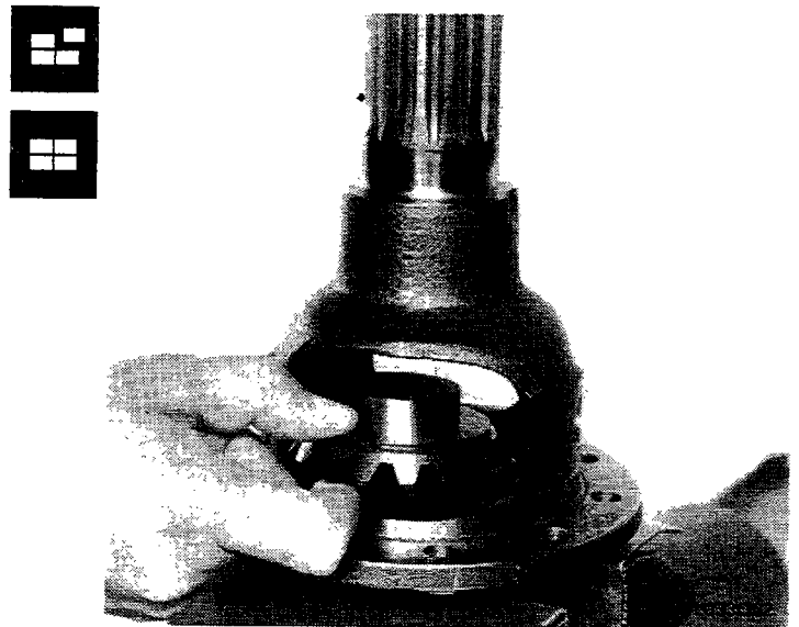
Removing-refitting planet wheels from differential casing
